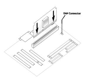
**Note:** G4 processor cards include a fan. If you own one of these cards, you must connect the fan with the appropriate fan connector on the mainboard as seen on the picture above.
