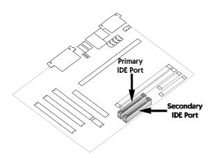
3. Connect an IDE cable on the back-panel of each IDE device to the corresponding headers on the mainboard. Close the tabs to secure the connector. Please note that IDE cables are directional and cannot fit correctly unless properly oriented.
